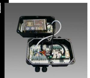
Waterproof gear box with LED FULLCOLOR power supply and DMX interface
