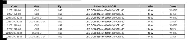
The reported luminous flux is the flux emitted by the light source with a tolerance of ± 10% compared to the indicated value. The W tot column indicates the total wattage absorbed by the system without exceeding 10% of the indicated
