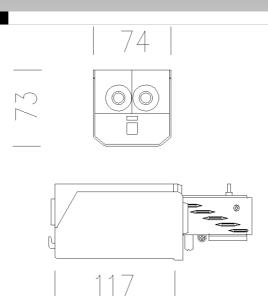
In nylon with phosphorous bronze contacts. To be used always to power the track. Maximum 2.5 sqmm permitted lead cross section  $\,$
